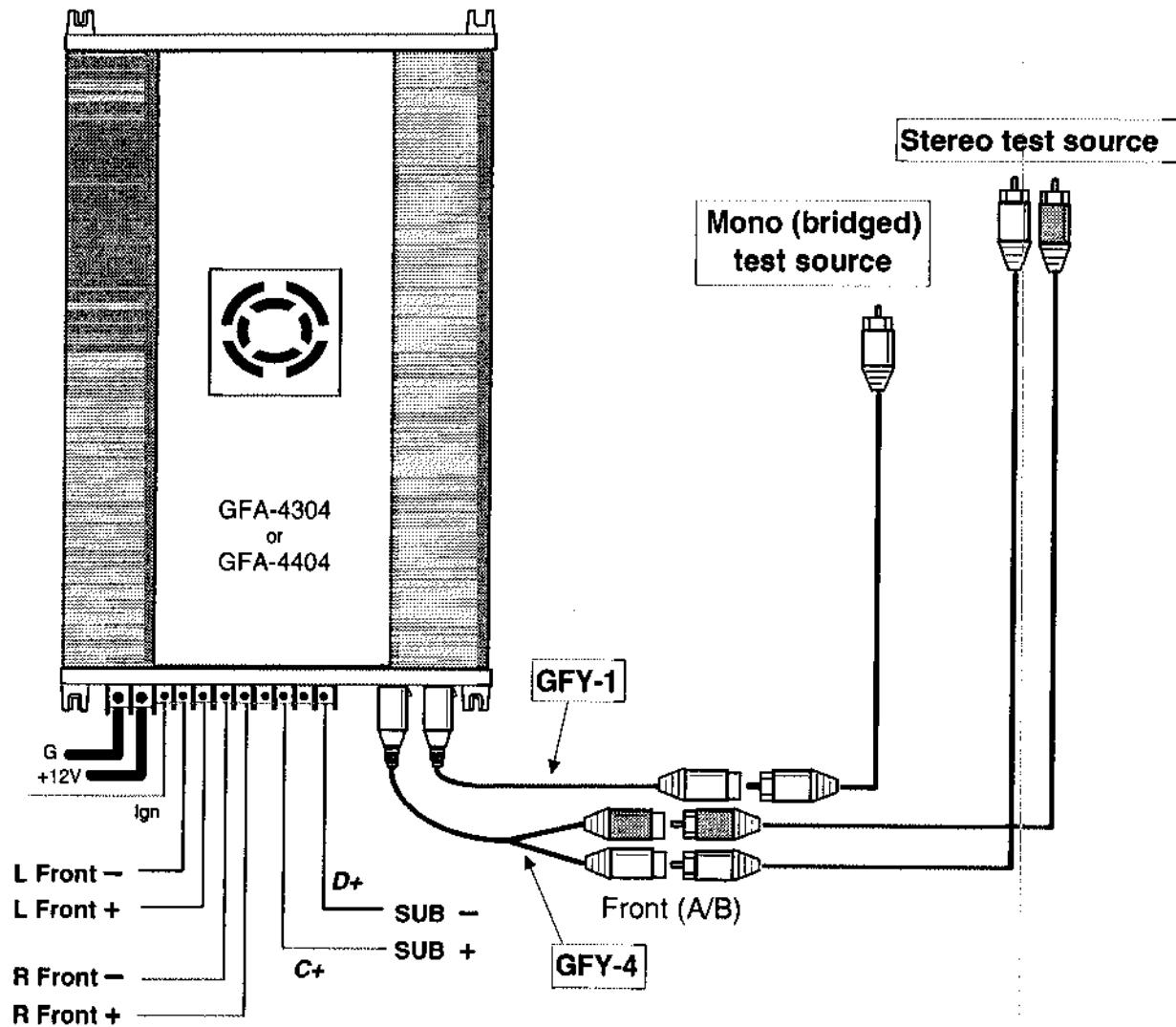
**APPLICATION:** Adapts XLR(2 ch.) input to accept mono RCA-type input and run amp in **MONO**
