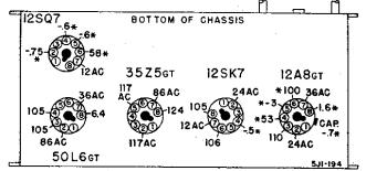
If taken with a 1000 ohm-per-volt meter, readings will either be lower or practically zero.
