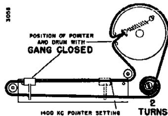
Dial stringing and pointer setting is shown with the gang condenser closed. The 1400 KC pointer setting is shown in dashed lines.
