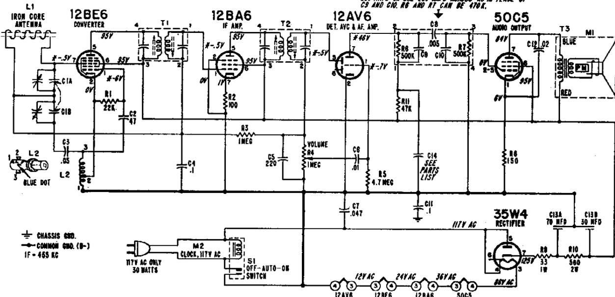
\*These voltage readings will be either lower or practically zero if taken with a 1000 ohm-per-volt meter.
