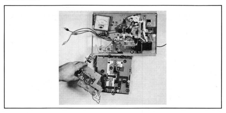
4. The board is now accessible to be worked on. Attach the red and black power supply wires to their appropriate connections.
