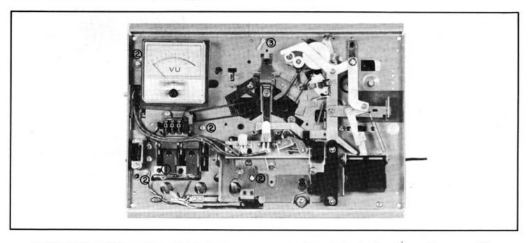
2. Pull wires through the slotted openings on the front of the PC board (3). In earlier models slots weren't provided therefore you will have to unsolder the wires and pull them through the holes. Lift transport up and swing in
