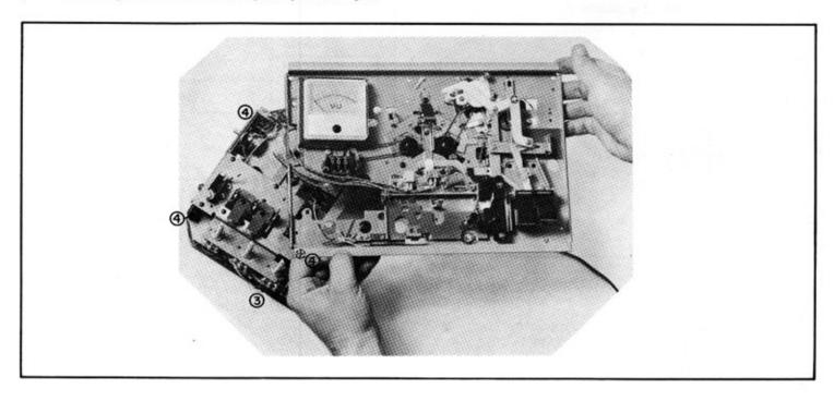
3. Remove 9 screws (all slotted 1-9) from the switch linkage (three of them with stand-offs) and place the top plate on the right of the PC board.
