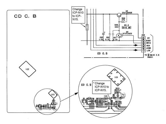
\* ICP-N10 is not described in the service manual. Instead it is described as jumper wire in the service manual.
