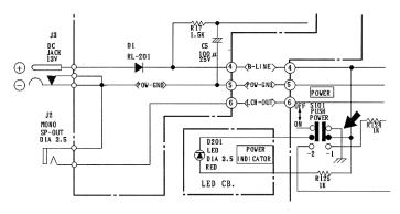
Solder flows into SW. When the power is OFF, +B flows into GND.
