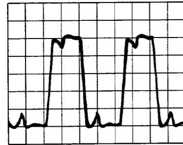
③ U2 Pin 18 (16.9M) VOLT/DIV: 1V TIME/DIV: 20nS
