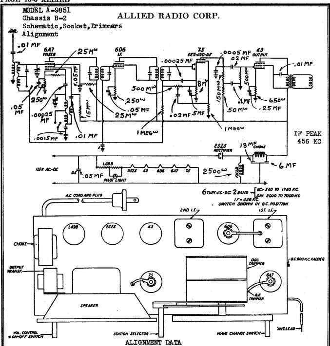
INTERMEDIATE FREQUENCY - Connect the Signal Generator to Grid of 6A7 tube through a .05 MFD. condenser. Ground Generator to Ground of Chassis. Set Generator at 456 KC and adjust Trimmers on IF Transformers for maximum peak.
