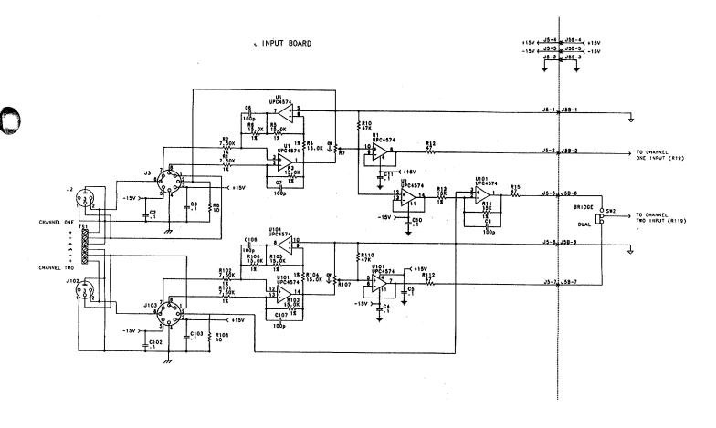
Figure 5. Schematic of Rear Input Printed Circuit Board
