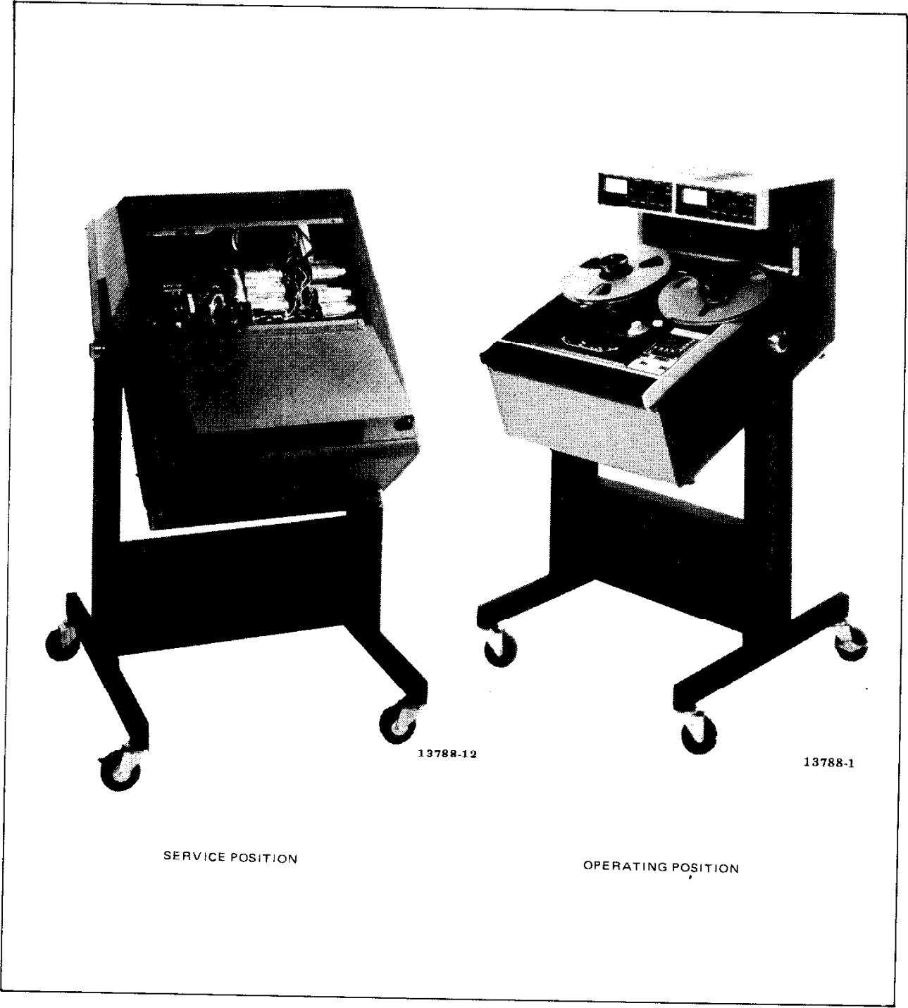
Figure 2-4. Cabinet Mounted on a Pedestal
