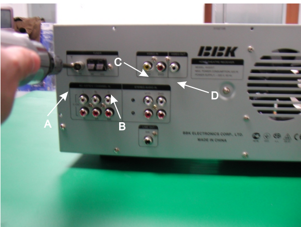
(13) Take hold of tuner by left hand, use electric screwdriver to fix screws A, B; take hold of video board by left hand, use electric screwdriver to fix screws C, D; insert flat cable respectively to proper position.
