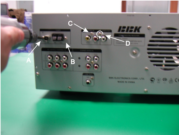
(5) Use electric screwdriver to unfix screws A and B in the joint position of tuner and rear cover, and then unfix screws C and D in the joint position of video board and rear cover, then take them down.
