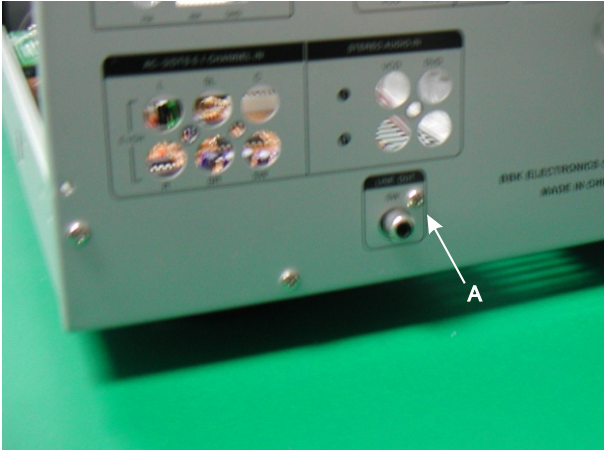
(9) Install signal board and use electric screwdriver to fix screw A of signal board.
