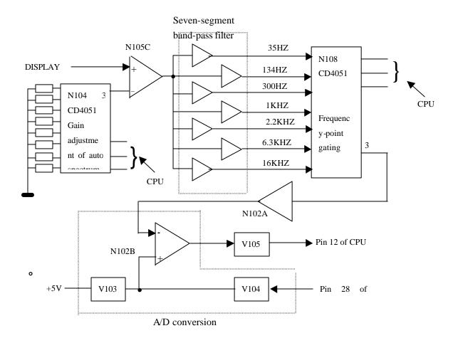
1, Automatic spectrum gain adjustment circuit: to avoid two situations that spectrum display amplitude is too low when input signal is too weak
