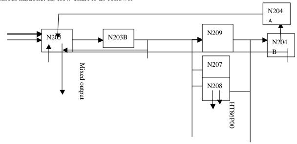
When pin 9/10 are of high level, sampled L/R/C signals are outputted via from pin 3 N205 gating, and sent to the internal of PT2399 after amplification by N203B for reverberation delay adjustment (by HT86P00 and HT86384 for voice processing), and then superposed to L/R/C channel to form different profiles.
