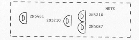
NOTE ORIENTATION OF TRANSISTORS AND IC'S IN SOCKETS
