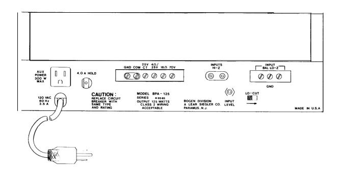
Figure 4 - BPA-125 Rear Panel Connection Diagram
