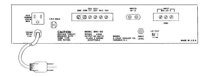
Figure 3 - BPA-60 Rear Panel Connection Diagram
