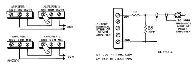
Figure 1 · Connecting Amplifiers in Series
