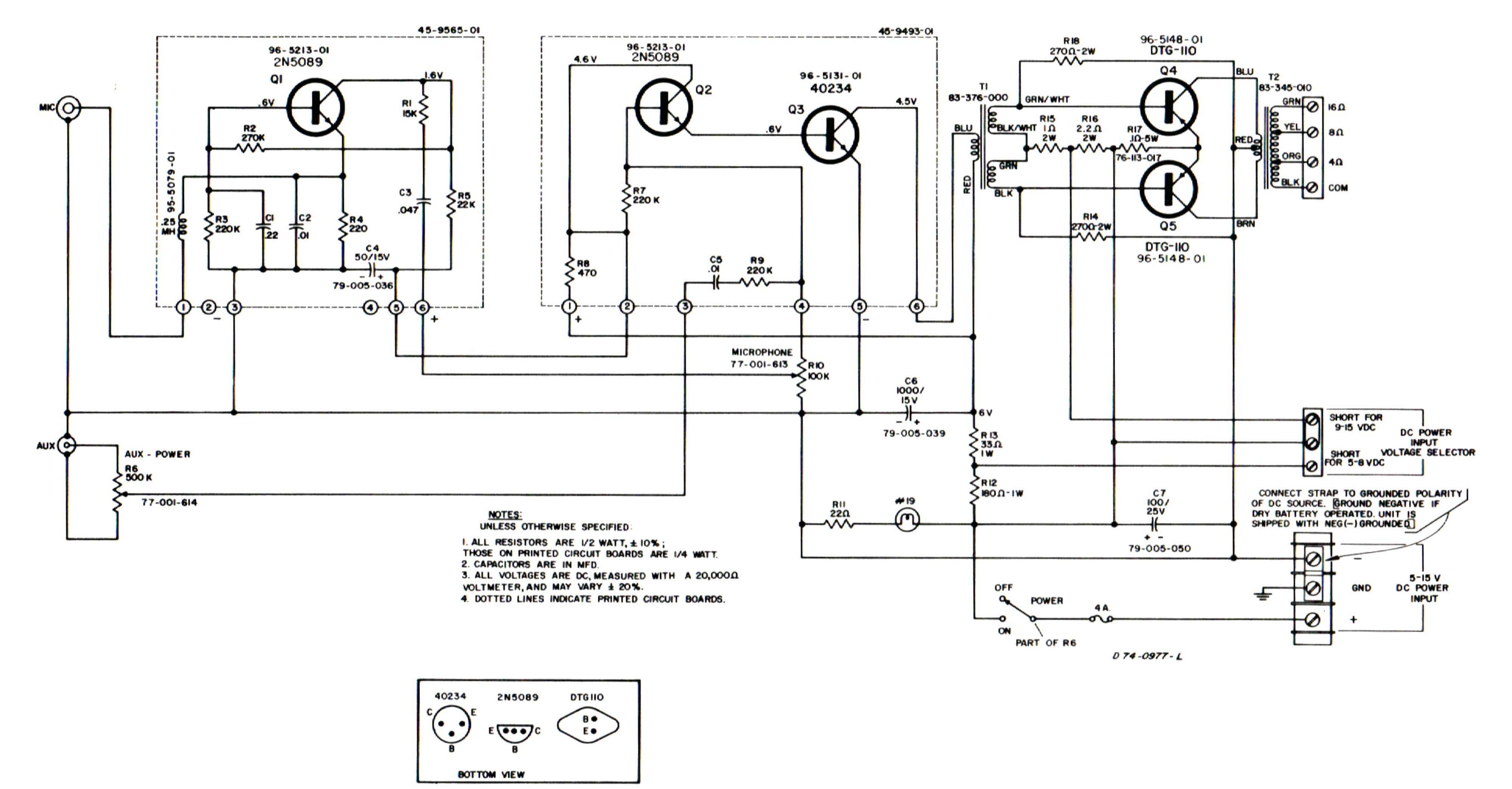
Figure 1-Model BT20A Amplifier, Schematic Diagram
