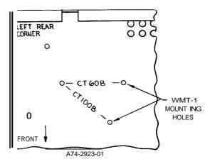
Figure 4 - Mounting Holes for WMT-1
