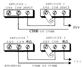
Figure 3 - Connecting Like Amplifiers in Series
