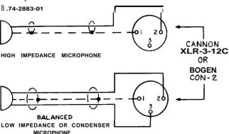
Figure 1 - Microphone Cable Connections
