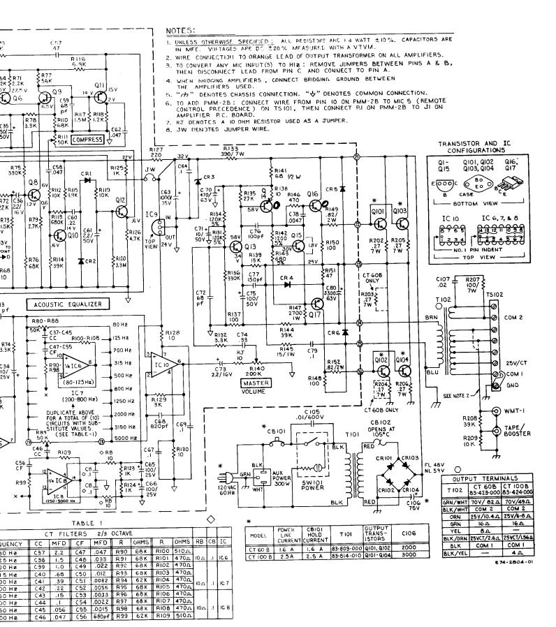
Figure 5 — Schematic diagram, Models CT60B & CT100B
