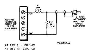
Figure 1 – Connection to Constant – Voltage P.A. Amplifier Driver.
