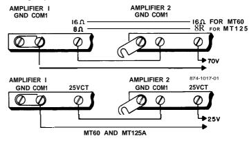
Figure 2 – Connecting Amplifiers in Series
