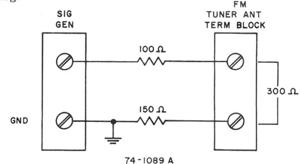
Figure 9 - FM alignment generator connections.
