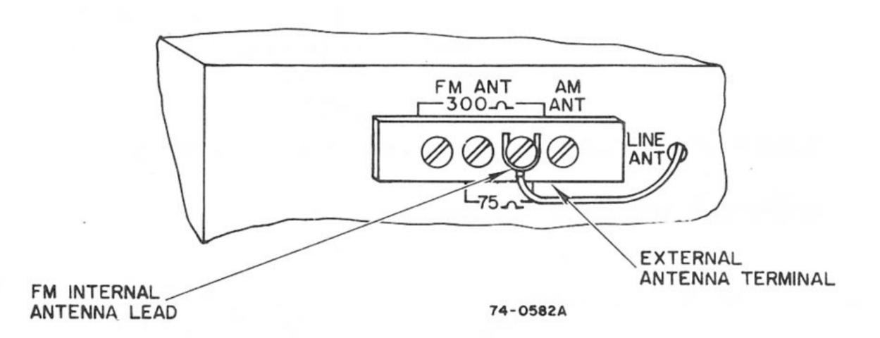
Figure 1 - Connection of FM line antenna.
