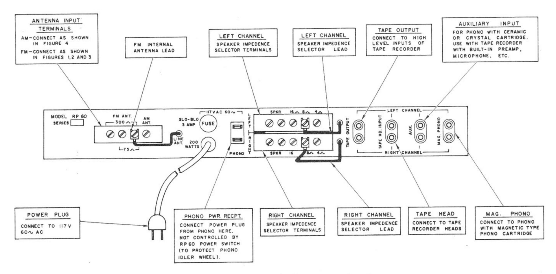
Figure 5 - Rear of chassis of RP60.
