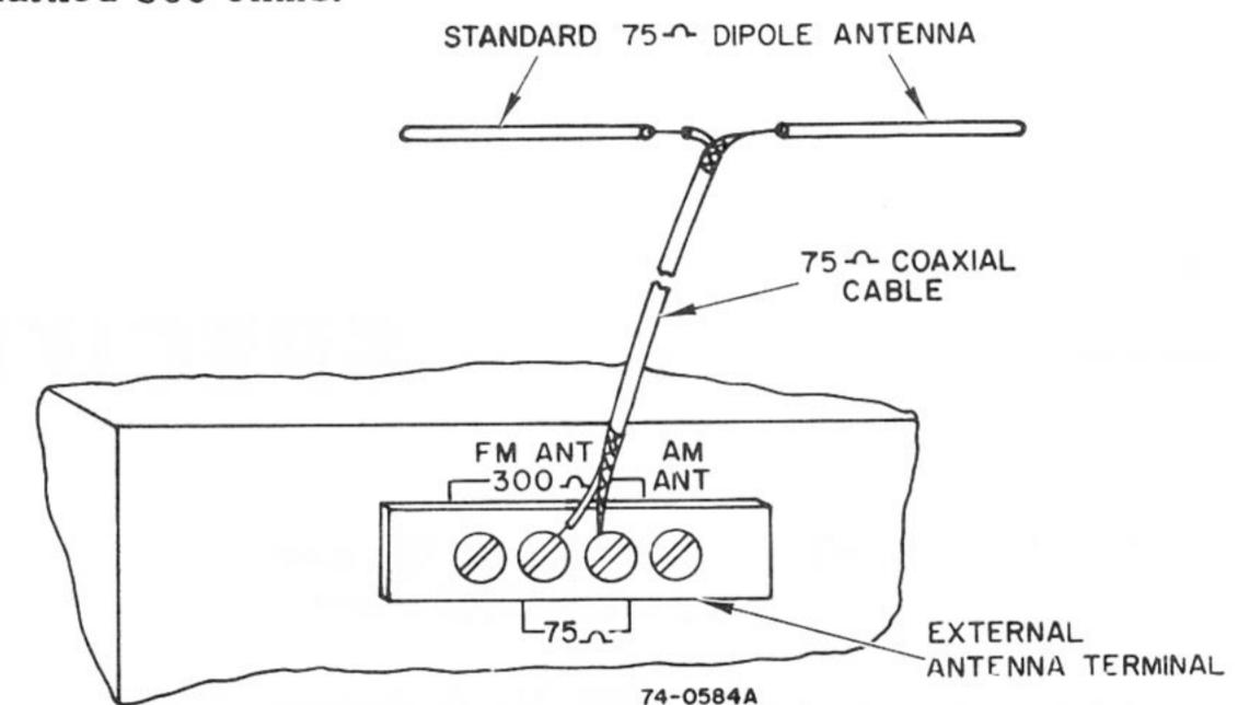
Figure 3 — Connection of external  $75\Omega$  FM antenna.
