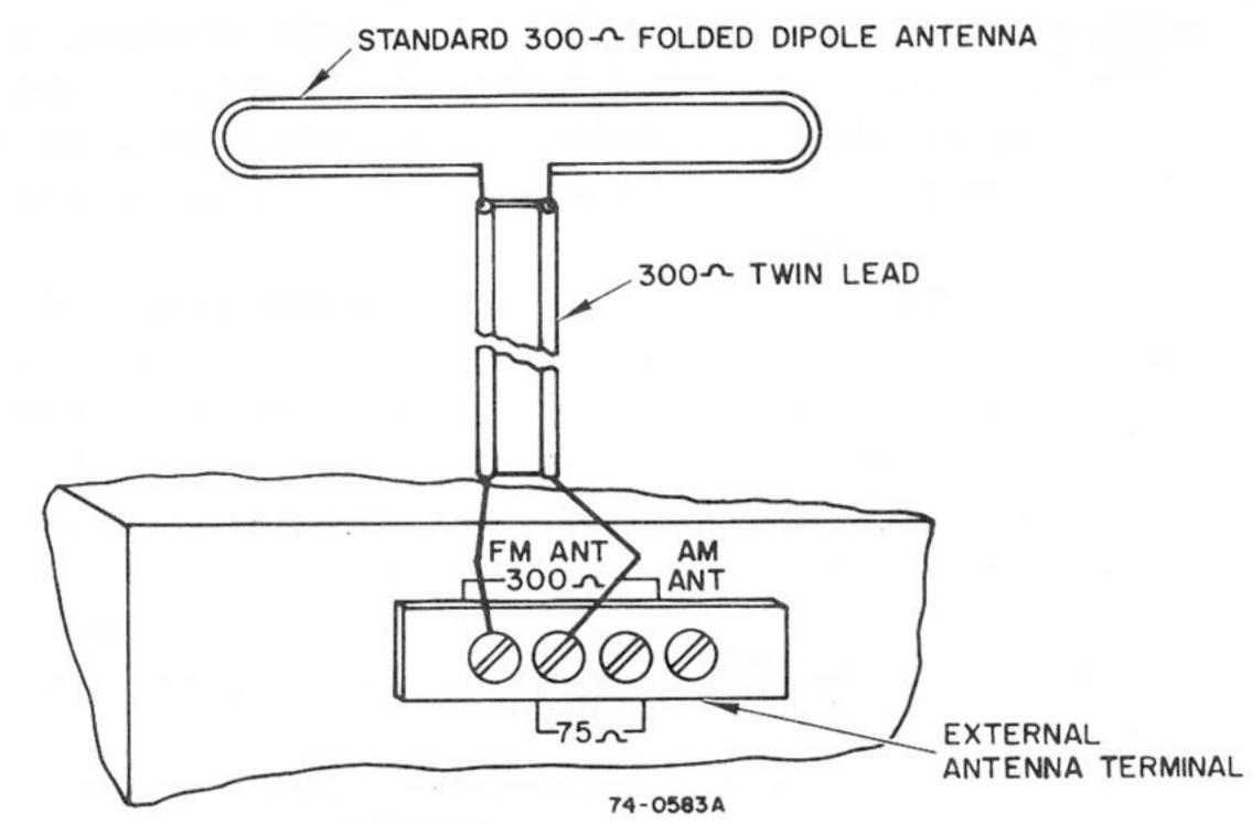
Figure 2 — Connection of external  $300\Omega$  FM antenna.
