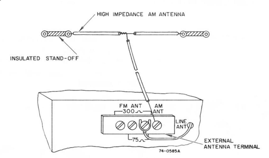
Figure 4 - Connection of external AM antenna.
