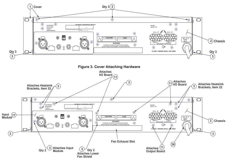
Figure 4. Rear View - Attaching Hardware
