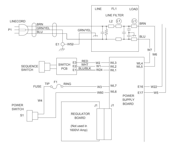
Figure 20. 1600VI and 1800VI 240V Wiring Diagram
