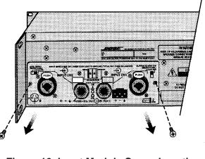
Figure 10. Input Module Screw Location
