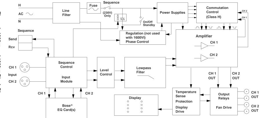
Figure 1. 1600VI and 1800VI Block Diagram
