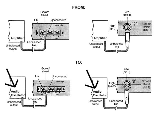
The input device was incorrectly identified as an amplifier. It should be a signal generator or audio oscillator.
