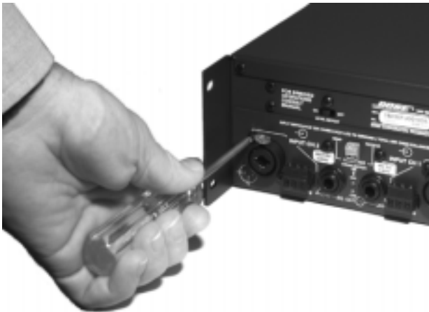
Figure 3. Input Module Screw Removal
