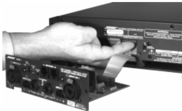
Figure 5. Amplifier Ribbon Cable Connector Location (ACM-1 J8 to amplifier J2)
