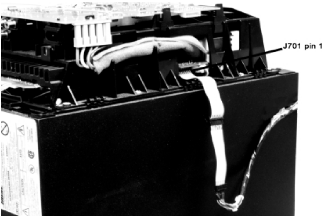
Figure 3. Output Wire Connection View at J701
