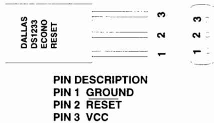
Figure 6. Pin Out IC DS1233
