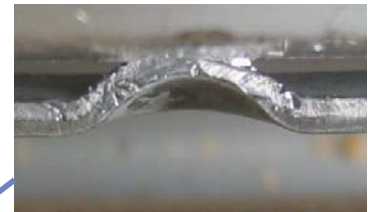
BEFORE Picture TAB barely under heat sink
