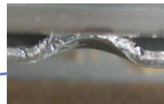
AFTER Picture TAB fully engaged under heat sink
