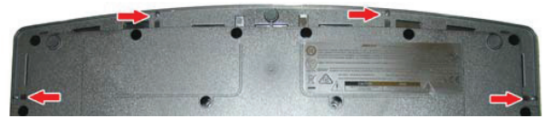
Figure 7. Metal Grille Screw Removal
