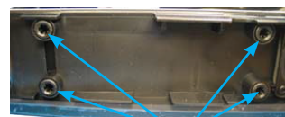
8 round grommets, 4 located on each side
