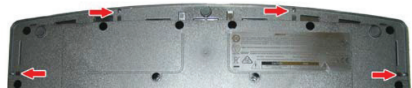
Figure 7. Metal Grille Screw Removal
