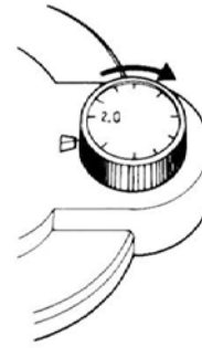
Fig. 9 Adjusting Anti-skate Control
