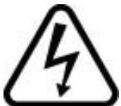
2. The lighting flash with the arrowhead within an equilateral triangle is intended to alert the user or service agent to the presence of dangerous voltages within the product enclosure that may be of sufficient magnitude to constitute a risk of electric shock to persons.
