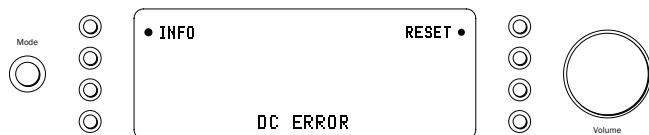
*Description* - CAP5 offers loudspeaker protection if the output of the amplifier goes to a high constant voltage (DC) because of some internal fault. This is a rare fault although detecting it could just save those expensive loudspeakers.
