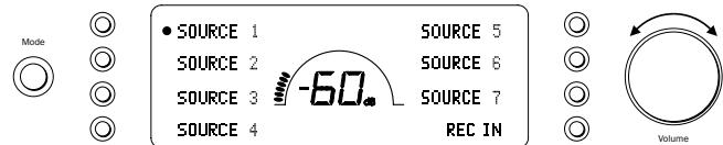
Adjust the volume control knob on the front panel (or using the remote control). The display will show the change in volume in decibels (dB). 'OdB' indicates maximum volume while lower volume settings progress into the negative range. This can also be changed to volume units (0-96) in the System Configure menu.
