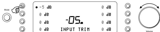
The relative levels of the inputs can be adjusted by gain trim. This allows each to be adjusted so that each sounds the same in terms of average loudness when you switch between them. Pick the loudest sounding source and trim its level until it matches the average perceived level of the others. Repeat this process if other sources also stand out as louder than the average.
