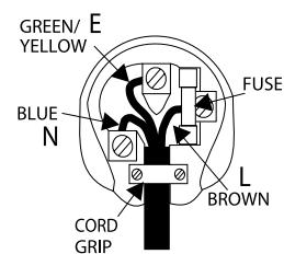
If a standard 13-amp (BS 1363) plug is used, a 5-amp fuse must be fitted or, if any other type of plug is used, a 5-amp fuse must be fitted, either in the plug or adaptor, or on the distribution board.
