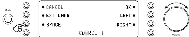
Press and hold the relevant input select button for four seconds to change its name. For example, if Input 1 is a CD player, name it "CD" etc. Letters are selected by turning the volume control to scroll through the available characters. Press LEFT or RIGHT to select which character you wish to edit. Press EXT CHAR to access an extended character set. Press OK to confirm and exit the input name change menu.
