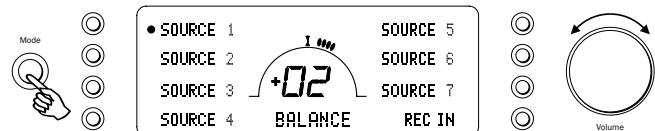
Press the Mode button to enter Balance mode. BALANCE will appear on the display and can be adjusted using the volume control. Press the Mode button again to return to Volume mode or wait 5 seconds for the 851A to automatically exit Balance mode.
