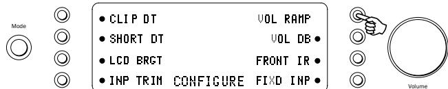
The 851A automatically ramps the volume down when going into Standby mode and up when coming out of Standby mode. To turn this feature off, press the VOL RAMP input select button in the System Configure menu and set to off. Press the Mode button to exit.
