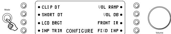
Press and hold the Mode button to access the System Configure menu. The menu options are Clip detector, LCD brightness, Speaker short detector, Input gain trim, Volume ramp, Volume display, Front IR and Fixed input gain.
