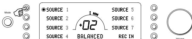
**Note:** To select the balanced input on either Source 1 or 2, repeatedly pressing the Source 1 or Source 2 button on the front to toggle these inputs between 'Balanced' and 'Unbalanced' source input.
