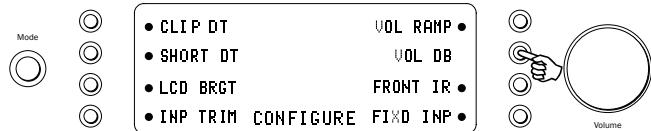
To change the volume display from decibels (-95 to 0dB) to arbitrary volume units (0 to 96 units) select VOL DB in the System Configure menu. Press the input select button to turn off the volume in decibels. Press the Mode button to exit.
