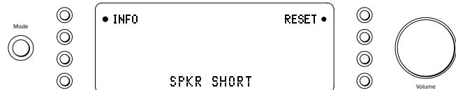
*Description* - During power up from Standby CAP5 performs a check on the loudspeaker terminals to see if a short across the terminals has been accidentally introduced (display flashes "SPKR CHECK"). If the resistance measured across the loudspeaker terminals is too low the unit will stay in Standby mode until the fault has been removed and Power up is re-attempted (display flashes "SPKR SHORT").
