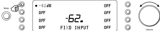
Select the input required and set the fixed gain using the volume control (the OFF setting does not disable the input but leaves the input gain subject to the volume control which is the default setting). When a source has a fixed input, the balance is always set to neutral. Press the Mode button to exit.
