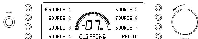
*Description* - CAP5 has the ability to detect when the amplifier starts to clip or overdrive at its output, which can damage loudspeakers, and degrade the sound. Clipping distortion is caused at high volume levels when the output signal attempts to go outside the maximum voltage that the amplifier can provide, causing the tops of the signal to flatten off. When CAP5 detects clipping the volume will be automatically reduced down until CAP5 detects an undistorted output.
