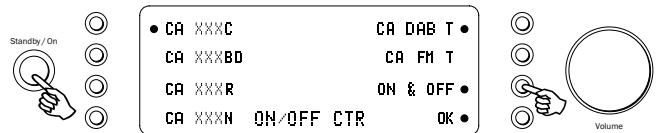
Select the connected Azur models by pressing the appropriate input select button. For example, CA XXXC for an Azur CD player (851C), CA XXXBD for an Azur Blu-ray player, CA DAB T for an Azur DAB tuner etc.
