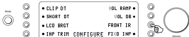
Used in conjunction with Custom Installation (C.I.) systems or IR repeater systems, it may be desirable to disable the front panel IR by setting FRONT IR to off (press the input select button to turn off). Press the Mode button to exit.
