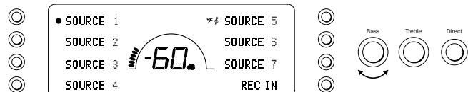
The 851A stores whether direct mode is on or off for each input individually, for example it is possible to have the tone controls automatically active for the Tuner source but not the CD source.
