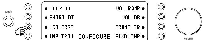
In the System Configure menu press the LCD input select button to scroll through bright/dim/off settings for the front panel display. Press the Mode button to exit.
