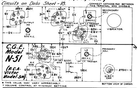
CONNECT CATHODE-RAY BETWEEN THIS TERMINAL AND CHASSIS. 60 Ð 1 Ø 0 6 g 260 K.C 0 ÖÕÕ I.F. TRANSF - 194V. (5) (B) (3) (B) VIBRATOR **(B**(R) O/,§5, C.G. 274V. 0V. **60** Mode/ PRIMARY ADJ. 0 © 🔞 260 K.C. I.F. TRANSF.
