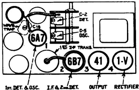
Model T4-2 is similar to Model T4-1 except for several modifications including: re-arrangement of wave-trap circuit, removal of oscillator low frequency trimmer, replacement of the 6F7 and 6A8 tubes with 6B7 and 6A7 respectively, and the reflexing of the I.F. stage for additional audio amplification. The I.F. remains at 460 K.C. The antenna and oscillator coils are aligned only at 1400 K.C.
