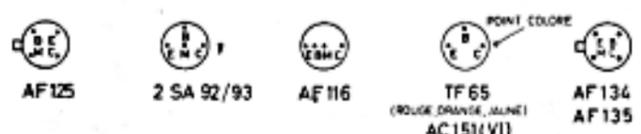
SUPPORTS TRANSISTORS (COTE SOUDURE) AC121(hb)
