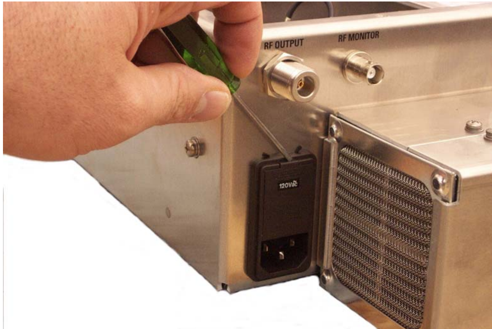
Illustration 2-1 Removing the Power Connector Cover
