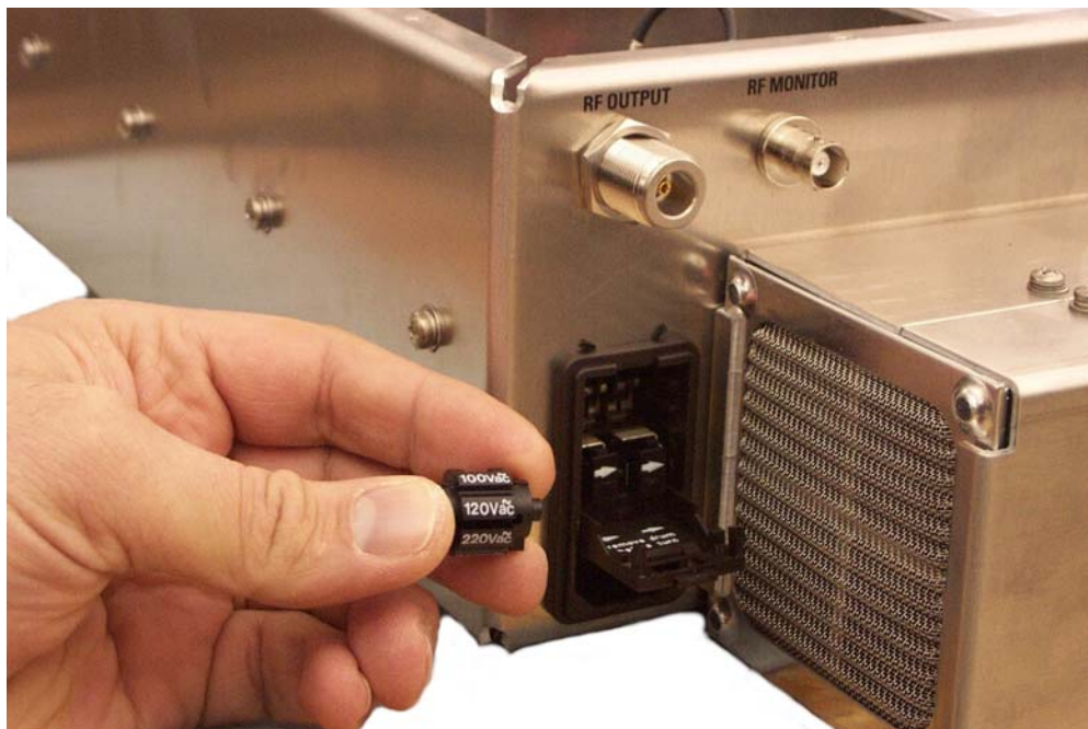
Illustration 2-2 Selecting an AC Line Voltage
