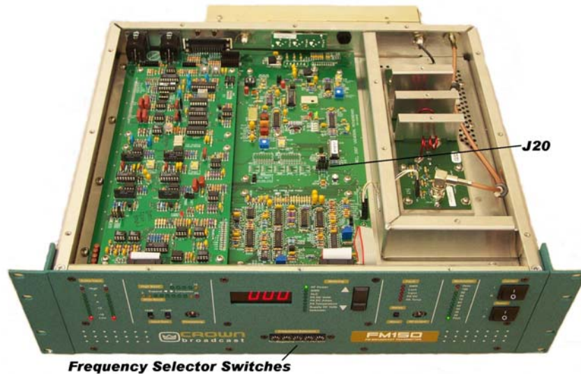
Illustration 2-6 Top Cover Removed
