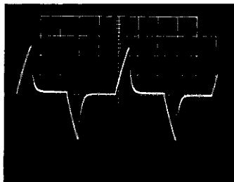
Fig. 7.5 Inductive Load Waveform, 2 ohms
