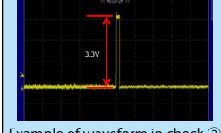
Example of waveform in check ② Voltage scale : 1.0V/div Time scale : 1us/div
