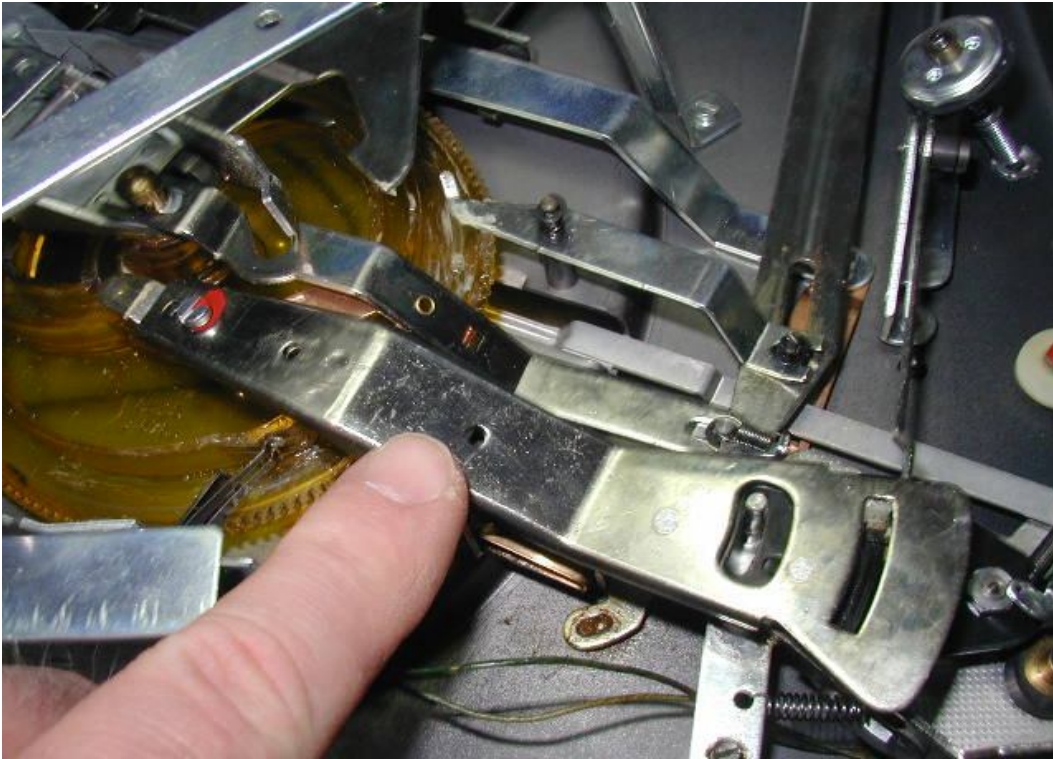
Hooked end of cueing lever in slot
