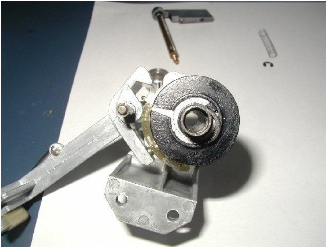
Large C-clip partially removed from pitch pointer...
