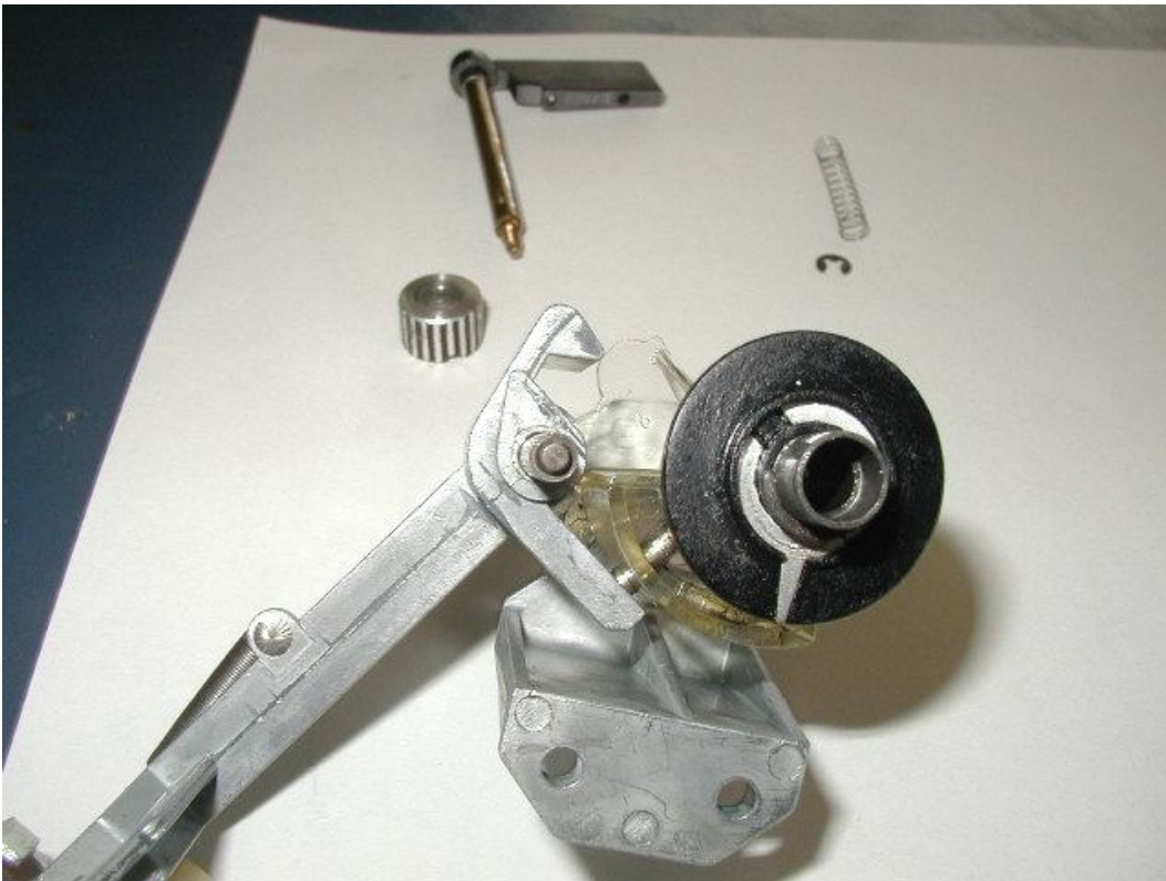
Speed control switch lever and pitch control knob removed-1219 2pc pitch knob.
