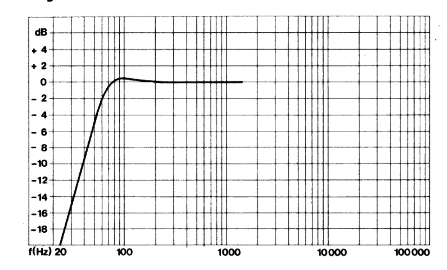
Fig. 8 Loudness control response O dB = volume control full gain
