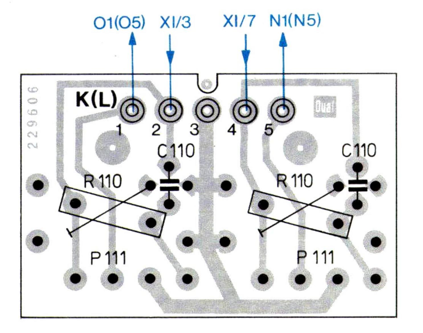
Fig. 23 Transformer connecting board, primary 229 603 (component side)
