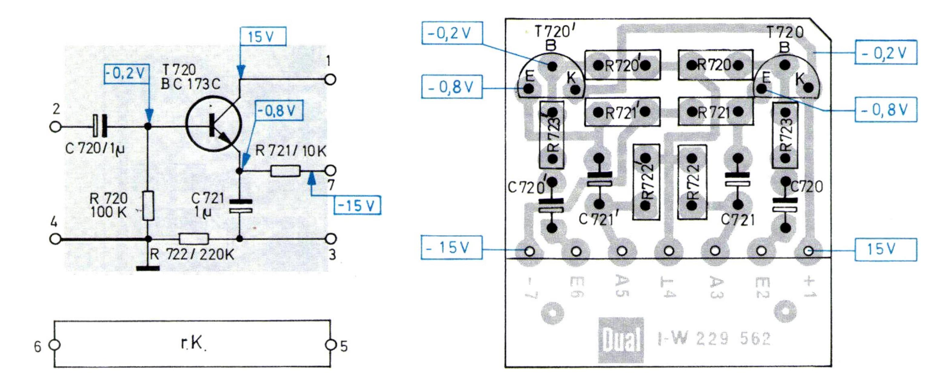
Intermediate amplifierVII Fig. 36 circuit diagram
