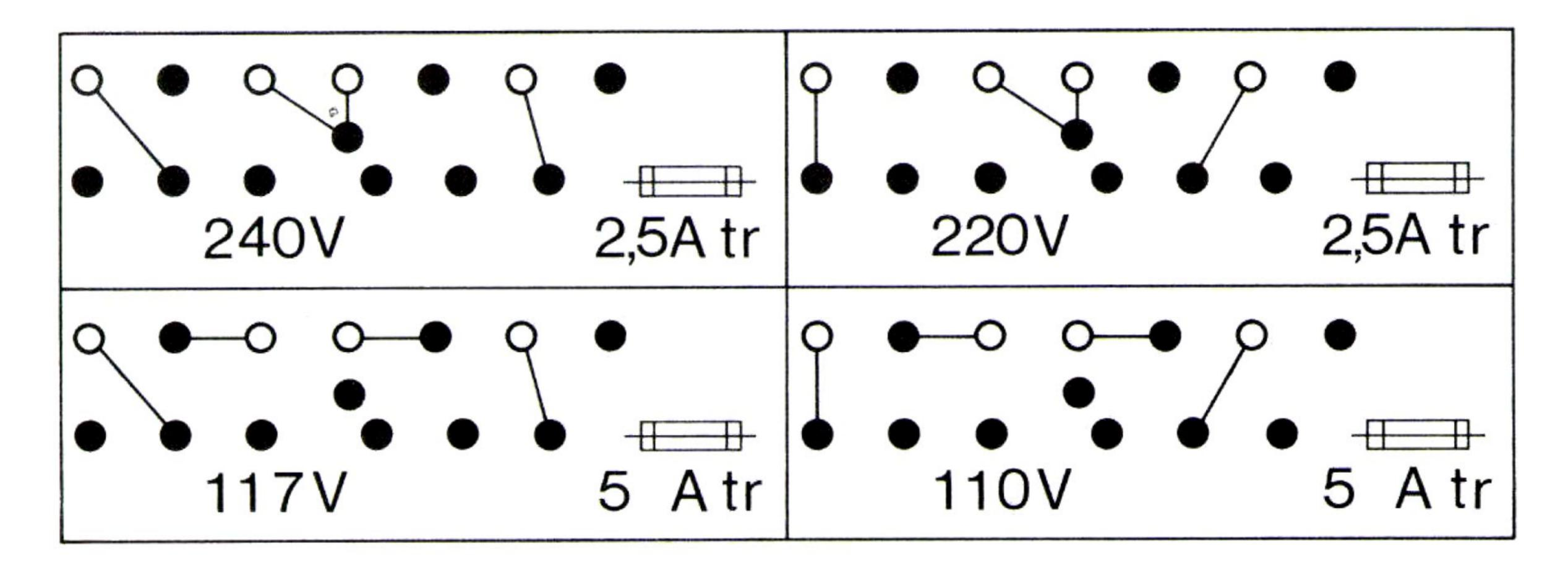
Fig. 25 Transformer connecting board, secondary 229 609 (component side)
