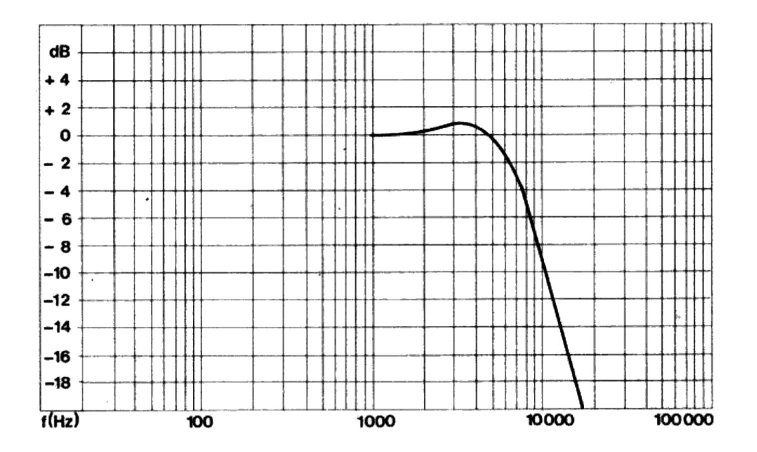
Fig. 7 Rumble filter response
