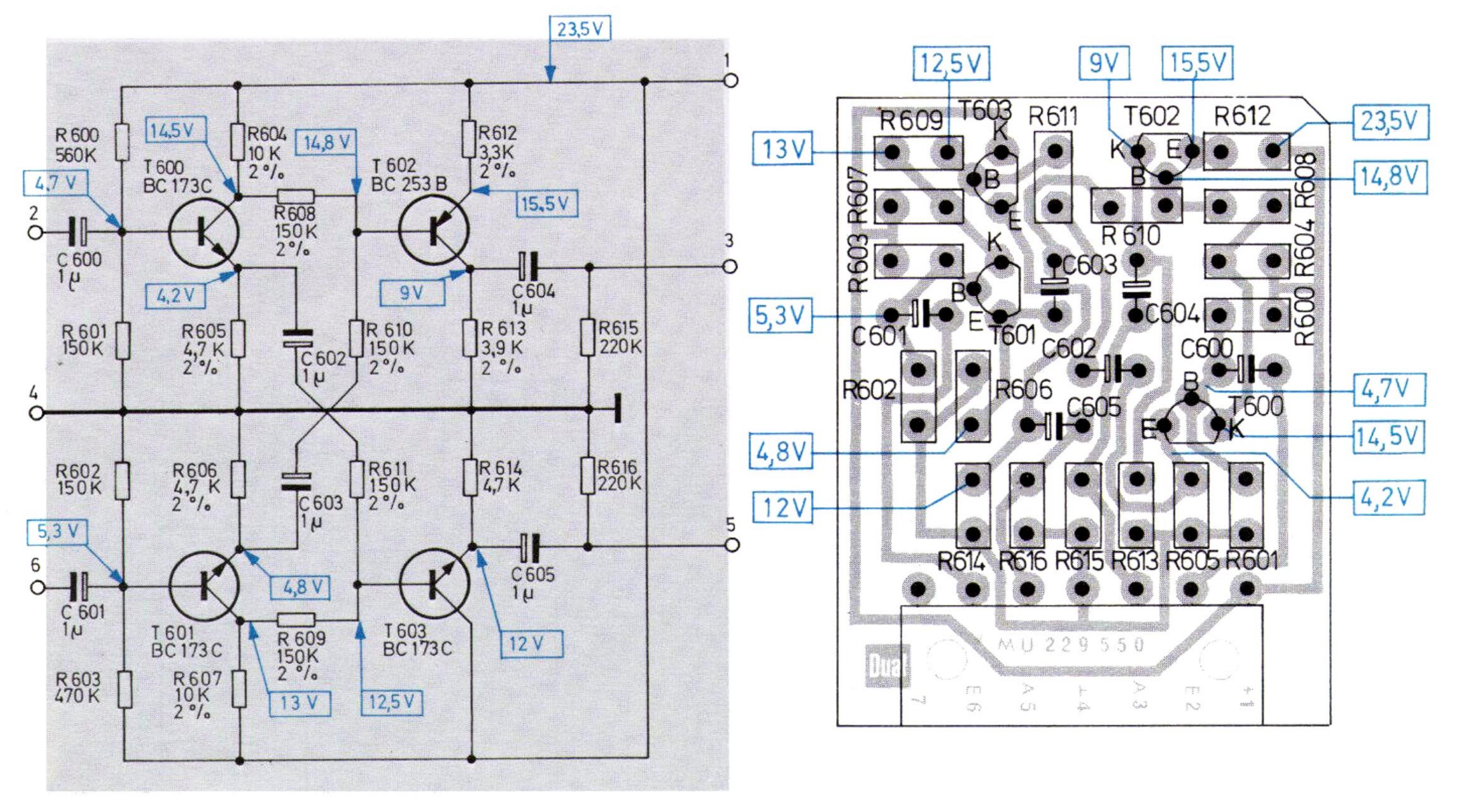
Fig. 32 IC amplifier V circuit diagram Fig. 33 IC amplifier 232 459 (conductor side)
