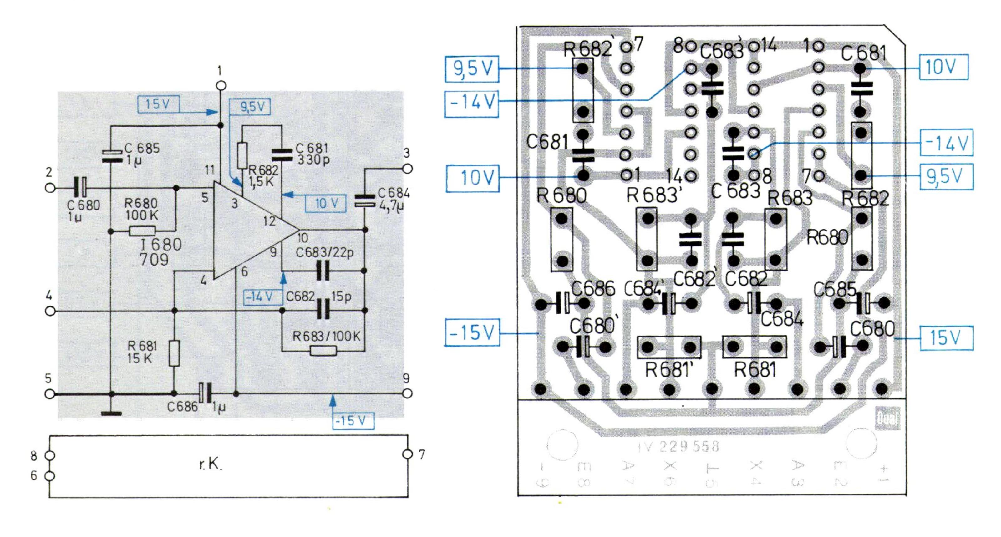
Impedance transducer VI Fig. 34 circuit diagram
