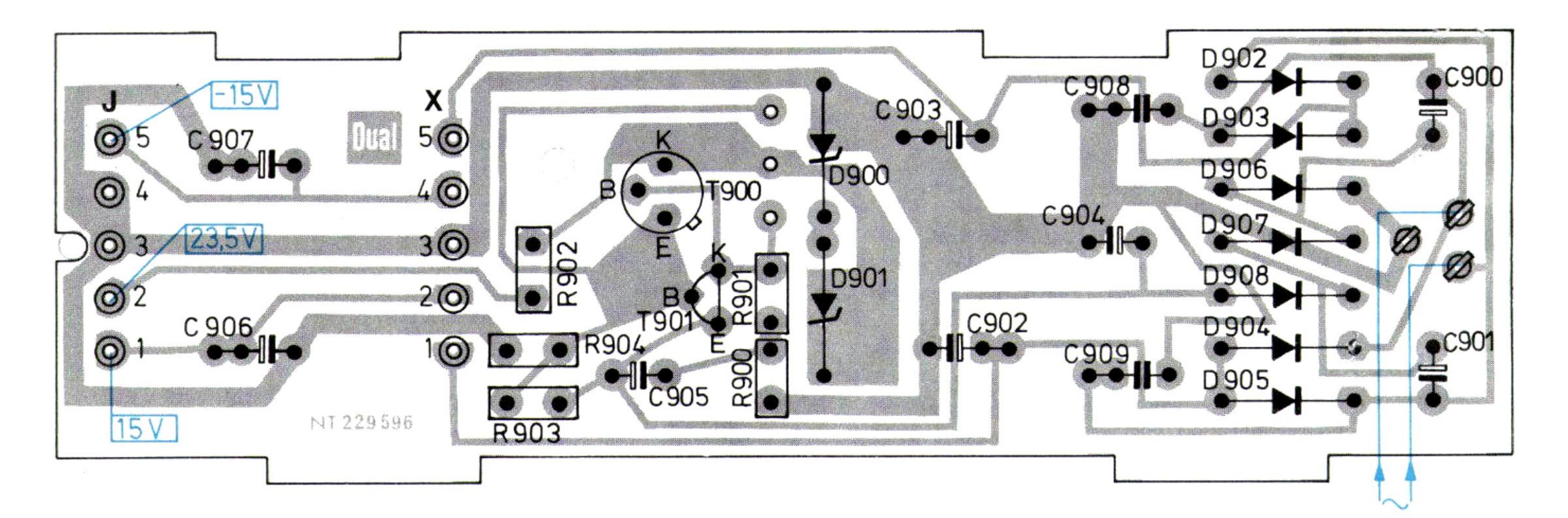
Fig. 44 Stabilizer X 233 057 (conductor side)
