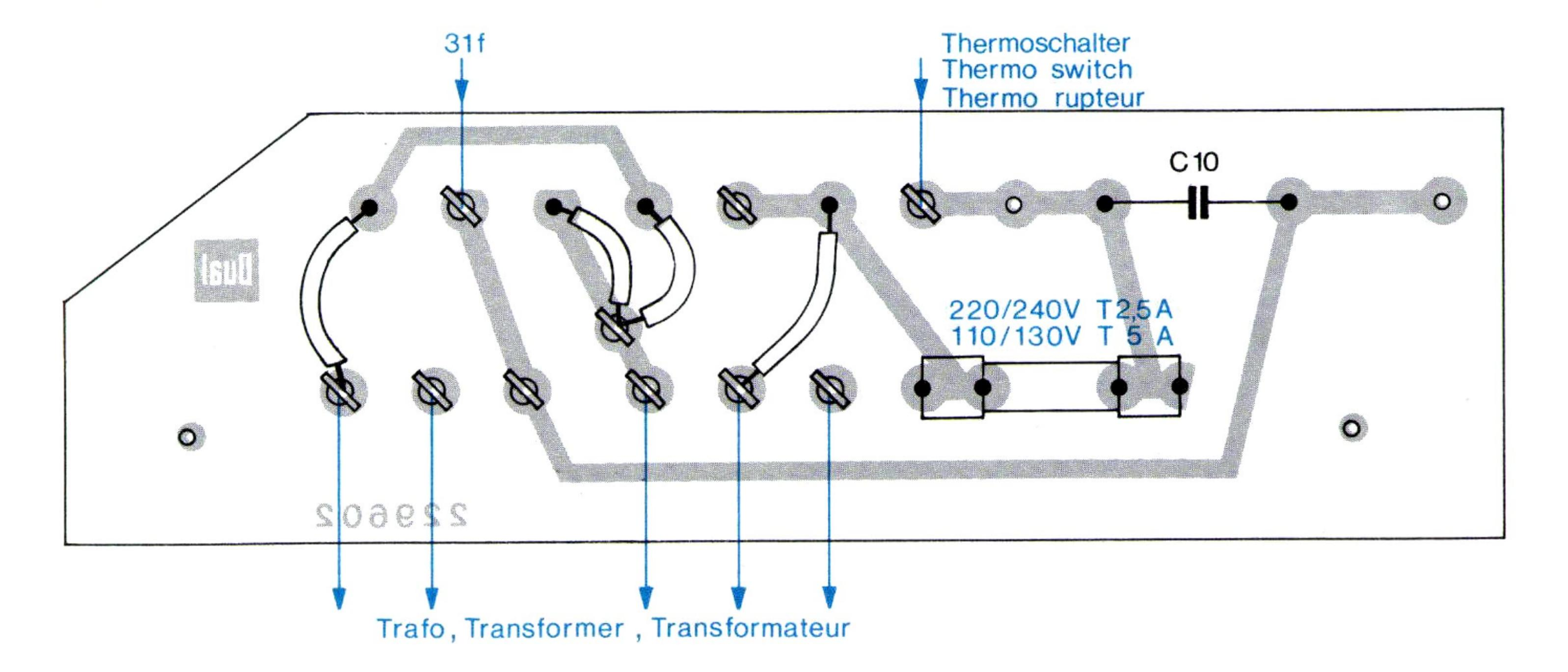
Fig. 24 Tapping scheme, 110, 117, 220, 240 V
