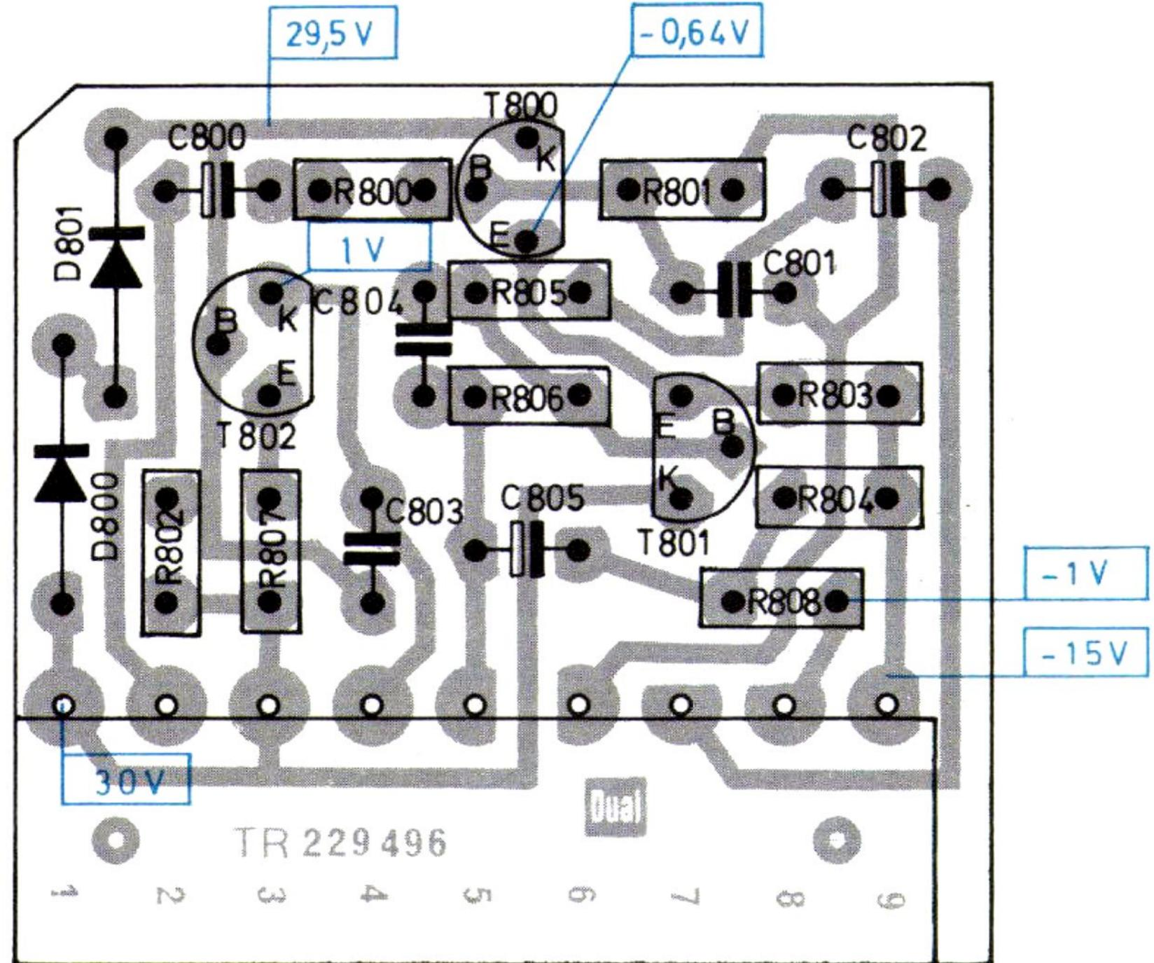
Fig. 40 Electronic fuse IX - circuit diagram
