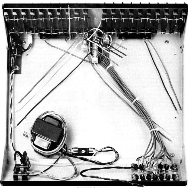
12( ) Select one conductor of the line cord, and connect it to outlet "B" lug #4 (S-2). Select the other conductor, and connect it to outlet "B" lug #3 (S-2).
