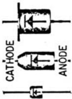
Connect the CATHODE lead of one of the rectifier diodes to lug #1 (*curved line symbol*) of the filter capacitor. Connect the ANODE lead to lug #2 of the 5-lug terminal strip (S). IMPORTANT: Arrange the diode leads exactly as shown in the pictorial diagram. When soldering,
