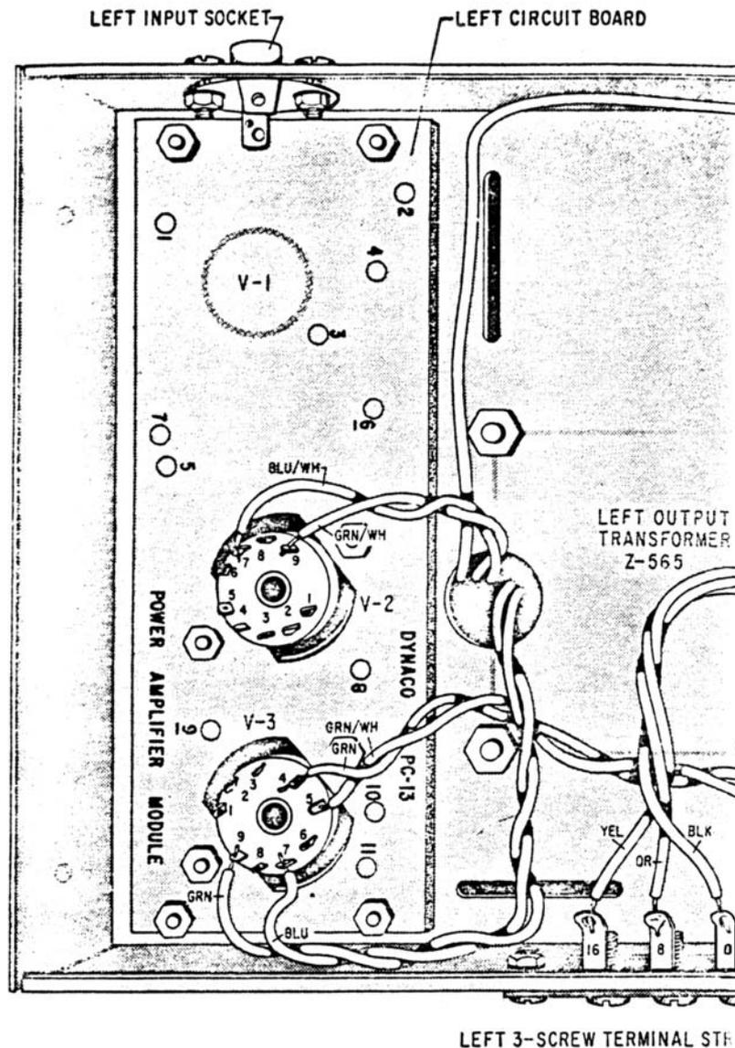
and-white leads from the LEFT output transformer to exactly 2" in length. Strip and tin the ends, and twist the leads together, as in the diagram. Connect the blue-and-white lead to pin #7 of V-2 on the LEFT circuit board (S).
