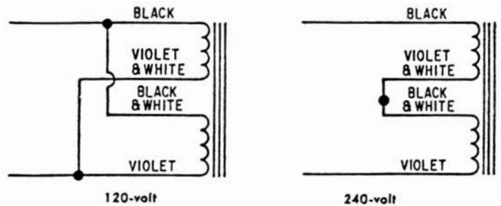
Dynakit Stereo 35 amplifiers supplied with power transformer PB-028 can be wired for use with either 120- or 240-volt a.c. power sources, in the following way:
