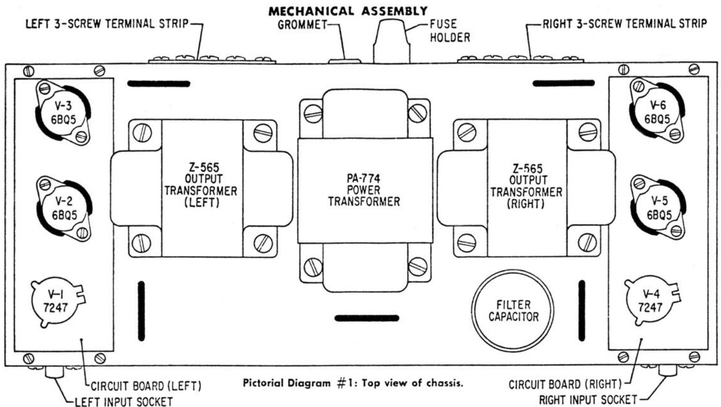
CHECK PICTORIAL DIAGRAMS #1 AND #3 BEFORE AND AFTER DOING EACH STEP.
