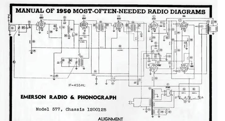
Volume control should be at maximum position; output of signal generator should be no higher than necessary to obtain an output reading. Use an insulated alignment screwdriver.
