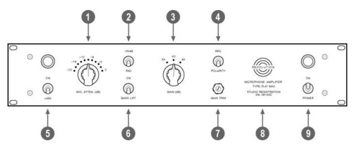
**1. MIC. ATTEN. (dB)** Eleven Position Input Attenuator Network (Pad) with a range from -20dB to 0dB in 2dB increments.
