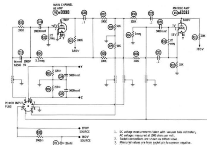
1. DC voltage measurements taken with vacuum tube voltmeter; AC voltages measured at 1000 ohms per volt.
