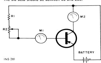
Voltage tests can be made with safety — without ruining transistors — by substituting resistors for the emitter-collector circuit of the power transistors. Voltages and resistor values are given
