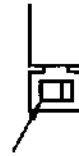
Fig. 2 Slide action of the switch will be sluggish if the hook protrusion is not centered but touching the side of the square hole.
