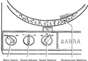
Motor Switch Speed Adjuster Speed Selector Strobe Diagram 1
