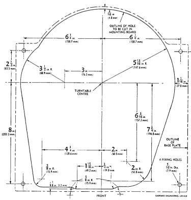
Reduced Template for Mounting Board. Diagram 8
