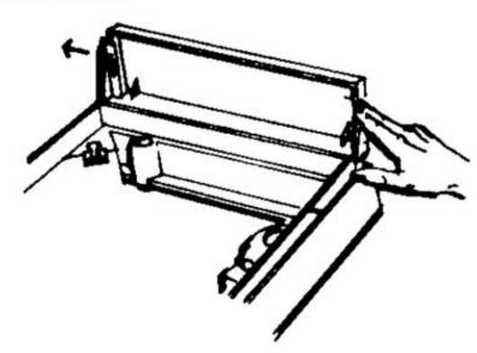
Mext, take the cover assembly and slide or place it on top of the base so that the 2 sides of the cover are aligned and sitting in the deep positioning grooves on each side of the Garrard base.
