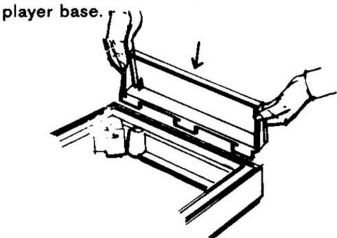
Press the panel down and slide to your left all the way, until resistance is met. The back panel is now rigidly locked into position. To remove, simply reverse the procedure.
