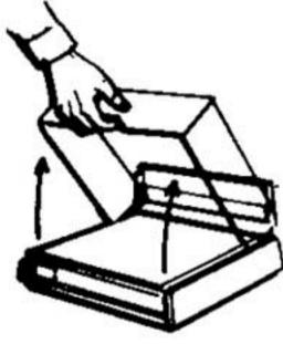
To raise the cover for loading records, unloading or adjusting controls, simply lift up on the front tab while applying gentle pressure backwards until the unique, self-aligning locking hinge assembly
