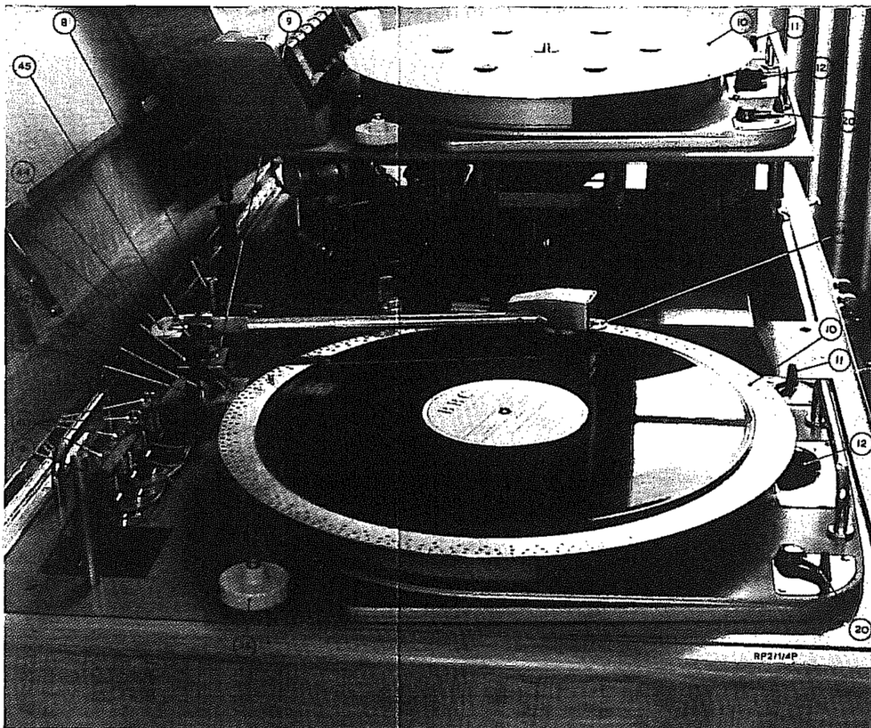
Fig. 4. Disk Reproducer RP2/1, Showing Pickup Arm RP2B/1
