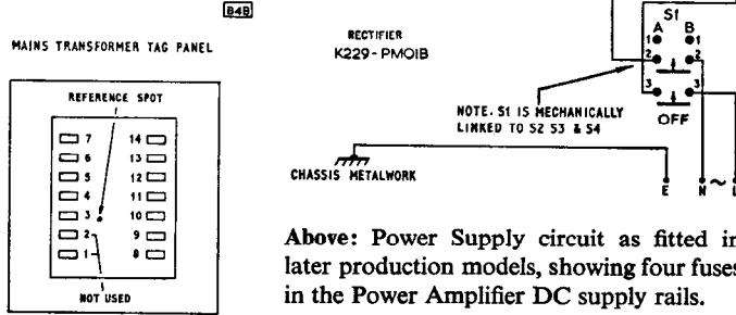
Above: Power Supply circuit as fitted in later production models, showing four fuses in the Power Amplifier DC supply rails.
