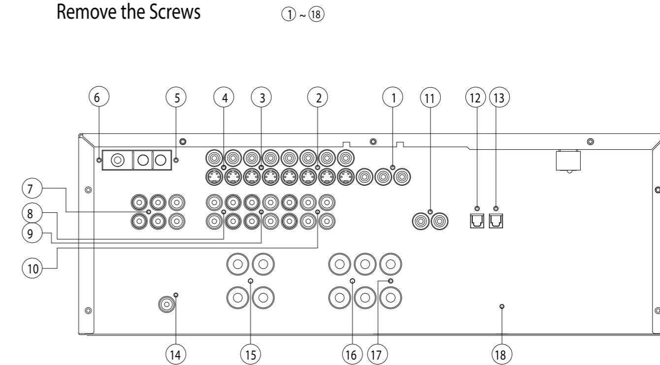
**4. Removing the Main PCB**
