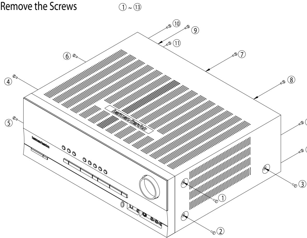
**2. Removing the Front Panel**
